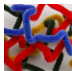
Rigid, contorted polymer chains cannot fill space
