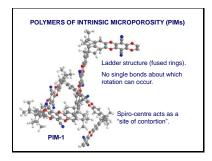
The backbone of PIM-1 is made up of little rings joined together.
