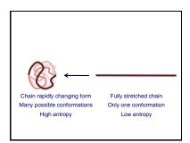
In the extreme of a fully stretched chain there's only one conformation; that's low entropy.
