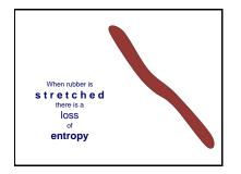
In modern terminology, the thermomechanical properties of rubber indicate that when rubber is stretched, there's a loss of entropy.
